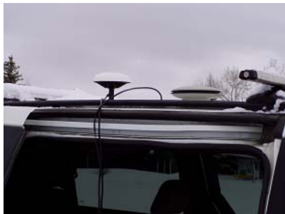
Figure 6. Antenna setup on the roof of the test vehicle
